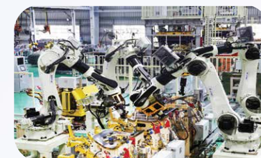
3. Body welding line
