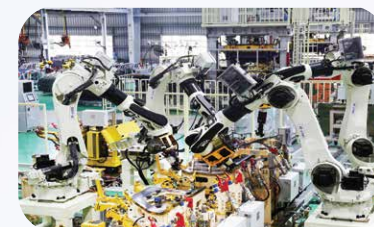
3. Body welding line
