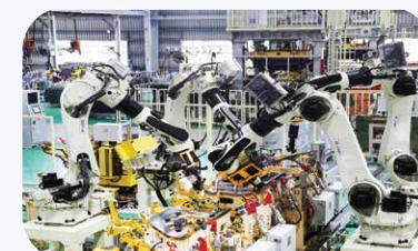
3. Body welding line
