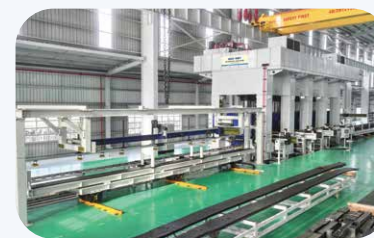
1. 1,600-ton stamping line for exterior sheet components of chassis beams.
