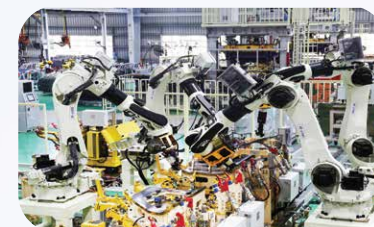
3. Body welding line
